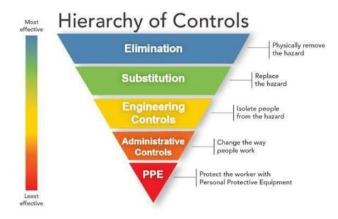
The idea behind this hierarchy is that the control methods at the top of the graphic are potentially more effective and protective than those at the bottom. Following this hierarchy normally leads to the implementation of inherently safer systems. Controlling exposures to hazards is fundamental to protecting our stakeholders through the organisations work place return during the current pandemic and its aftermath.
